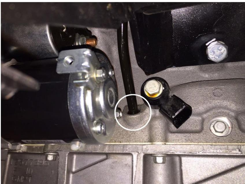
5. Fit the new pickup checking to make sure the o-ring is fitted and seals snugly when installed
