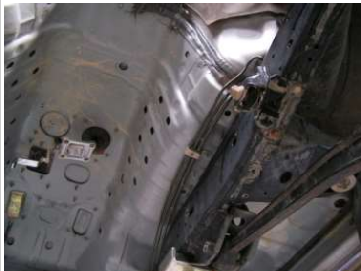
Image 1.2 Relocate fuel lines and rear brake pipe
