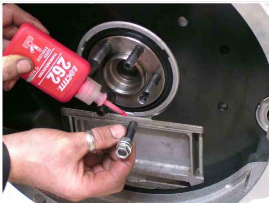
Image 3.1 Fit studs with Loctite
