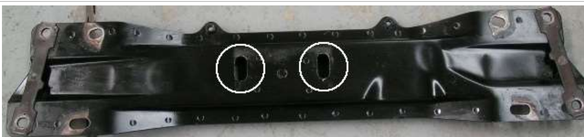
Image 1.7 Slot transmission rubber to cross member holes
