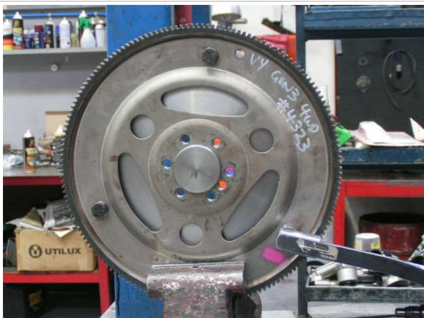
Image 4.2 Bolt flex plate to flywheel
