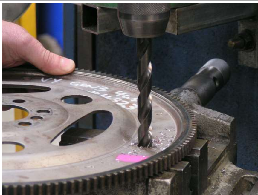
Image 4.1 Drill out the elongated hole to 12mm
