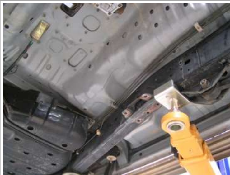
Image 1.1 Relocate fuel lines and rear brake pipe
