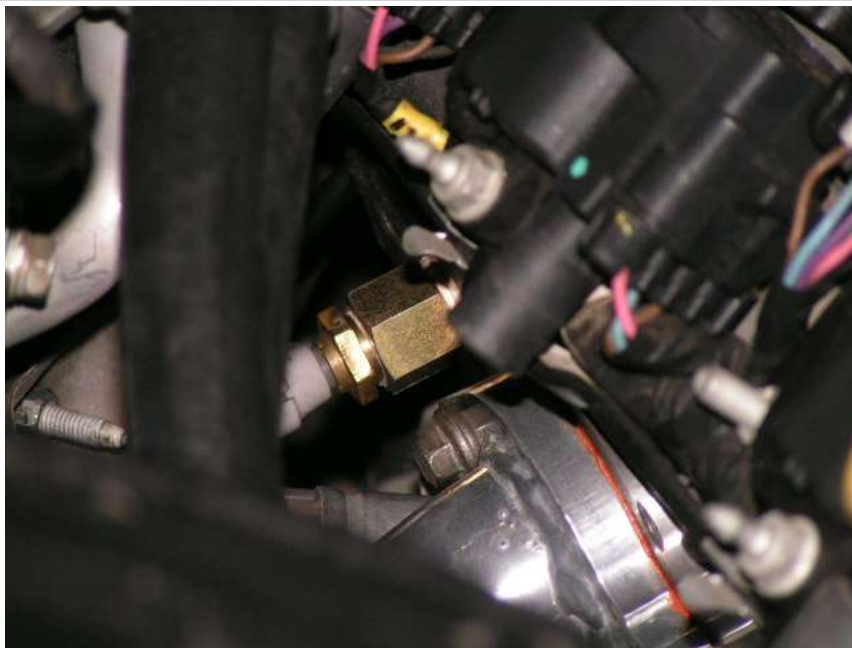
Image 1.6 Fit Adaptor (be carefull not to break off in head) and sender
