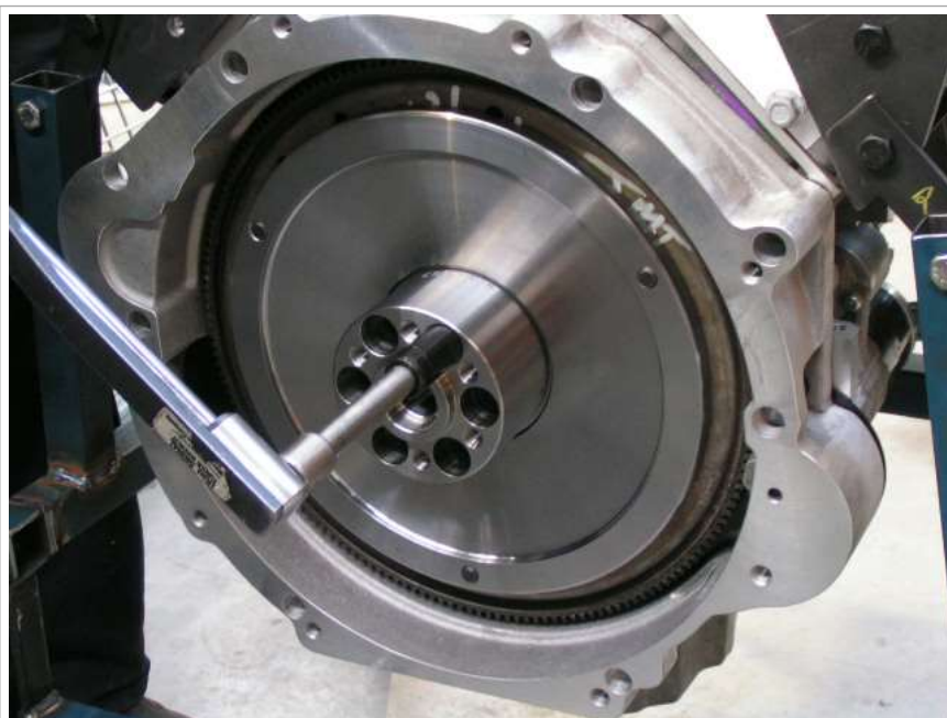
Image 4.3 Bolt flywheel adaptor on
