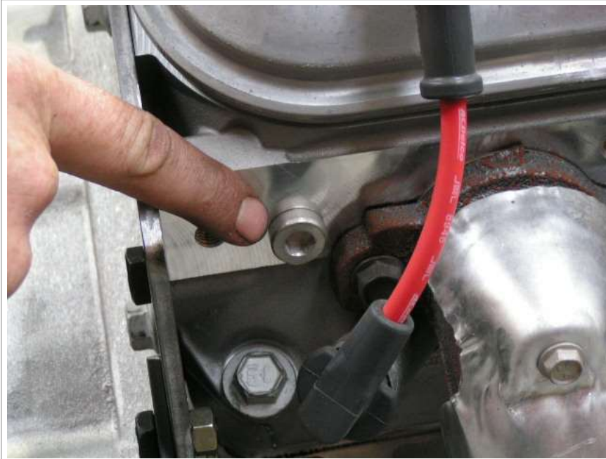
Image 1.5 Remove plug from head
