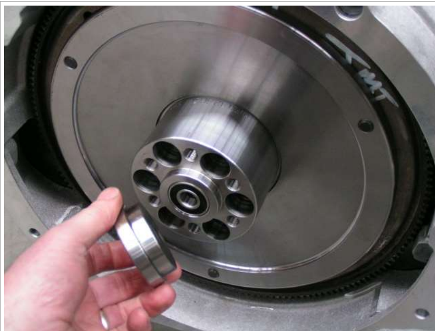
Image 4.5 Install spigot bearing
