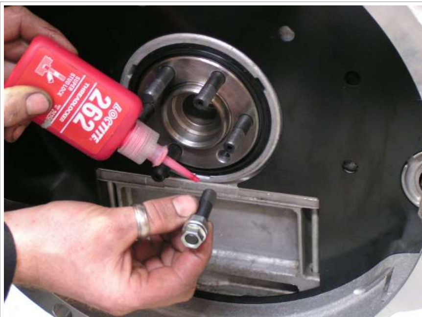
Image 3.1 Fit studs with Loctite
