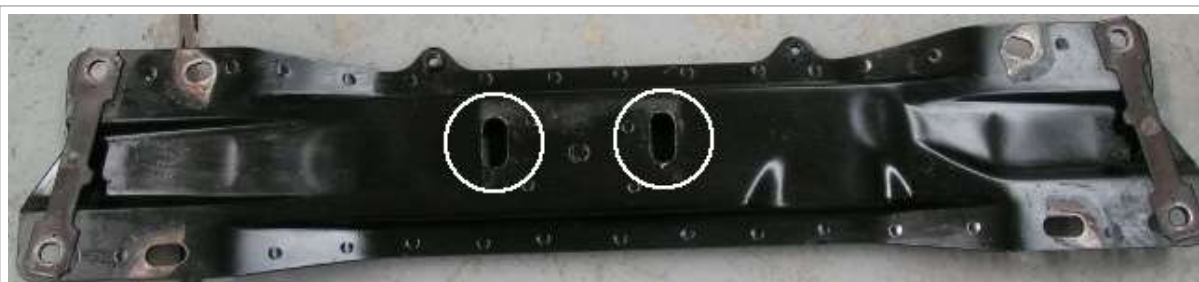
Image 1.7 Slot transmission rubber to cross member holes
