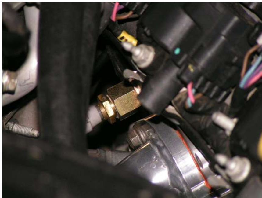
Image 1.6 Fit Adaptor (be carefull not to break off in head) and sender
