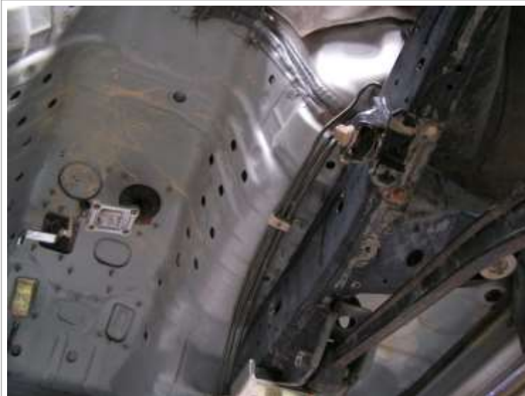
Image 1.2 Relocate fuel lines and rear brake pipe
