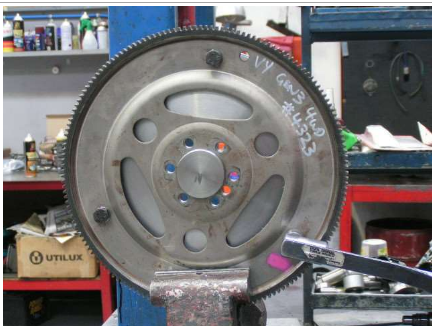
Image 4.2 Bolt flex plate to flywheel
