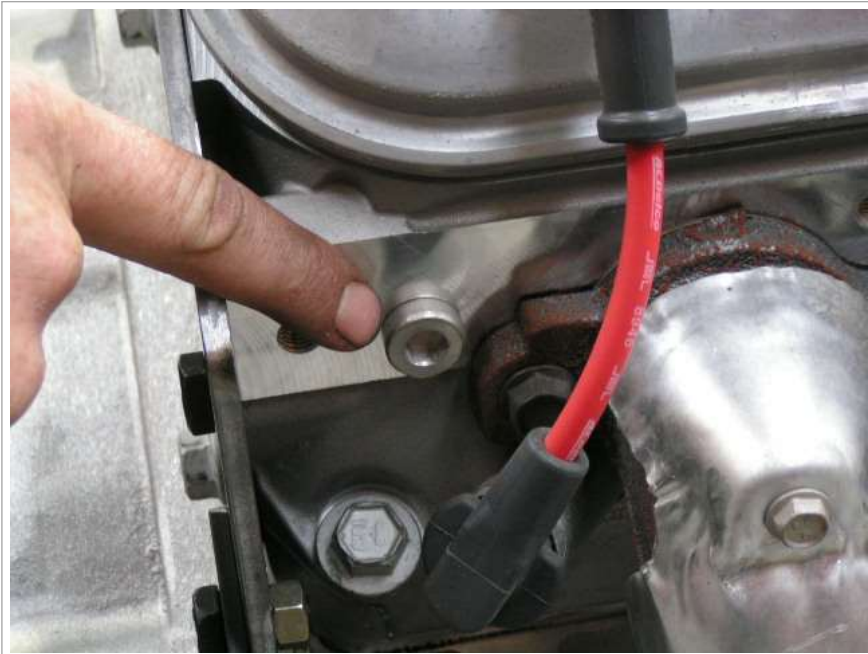
Image 1.5 Remove plug from head
