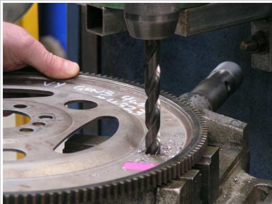
Image 4.1 Drill out the elongated hole to 12mm
