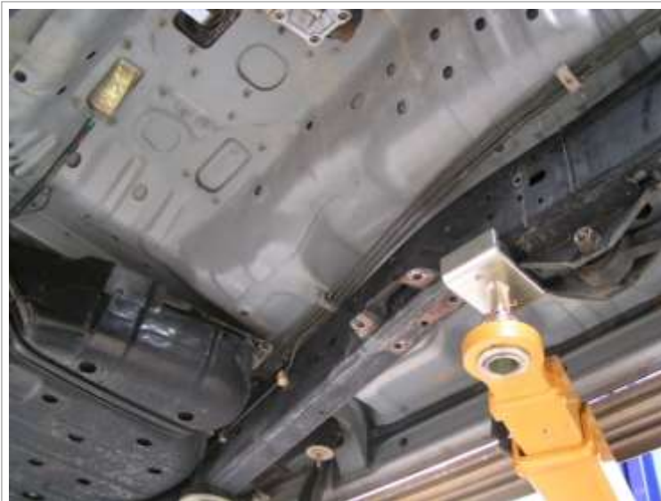
Image 1.1 Relocate fuel lines and rear brake pipe
