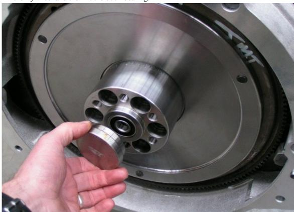
10. Fit the flywheel to the crank adaptor and secure it using the bolts supplied in the kit. Use
