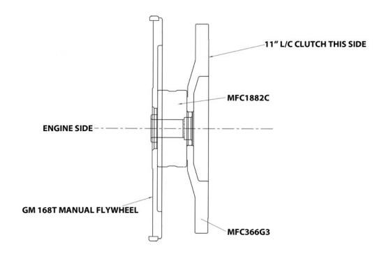
Fit the GM Chev Diesel manual flywheel to the engine, then the crank adaptor and secure it with the 6 socket head cap screws supplied. NOTE: PLEASE CHECK! the crank depth to make sure that the socket head cap screws do not bottom out). GM engines were fitted with various rear main seal types, the flywheel to crankshaft bolts/ socket head cap screws can touch in some applications. To prevent this a flat washer could be used under the head of the bolt. Use loctite on all crankshaft/flywheel bolts.
