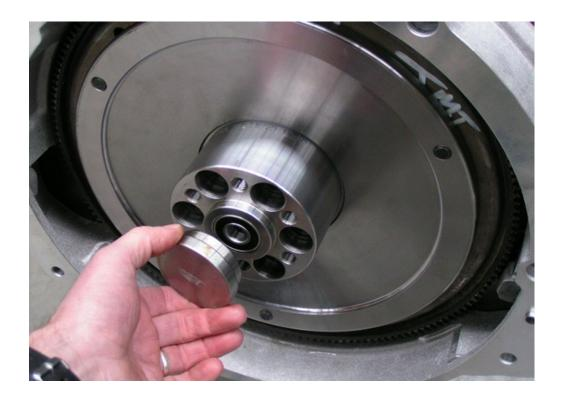
Fit the flywheel to the crank adaptor and secure it using the bolts supplied in the kit. Use loctite on all crankshaft/flywheel bolts.
