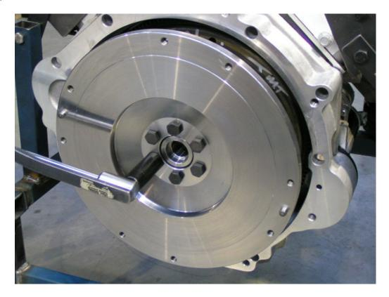
Make sure the dowels are fitted to the flywheel, they are required for correct clutch location. 3 for 1HZ and 2 for 1HDT
