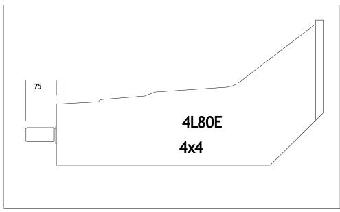
The diagram above shows the output shaft stickout length of a 4x4 transmission for which the kit was designed to fit without any modification.
