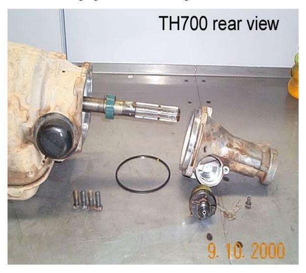
35. Next the output shaft will need to be cut down. Pack a rag into the back of the transmission around the output shaft to prevent any metal filings from entering the transmission while cutting the shaft.
