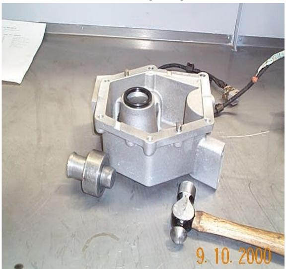
33. Fit the new seal (TC12586) in the back of the adaptor housing (MFC1195A) with the spring facing the transmission. *NOTE:* Use a suitable drift to fit the seal.
