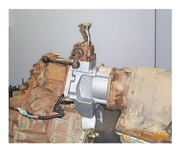
41. Fit the transmission assembly to the transfer case and secure it using the original Toyota bolts.
