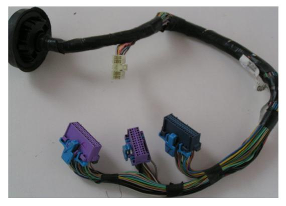
2. Mount the switch in a suitable location insuring the loom will reach the 9-pin connector. **NOTE:** If you have purchased an interface harness with the diagnostic light kit you will now have 2 of the mating plugs, obviously only one will fit. Put all of the relevant wires into one of the shells and discard the other.See the photo above:
