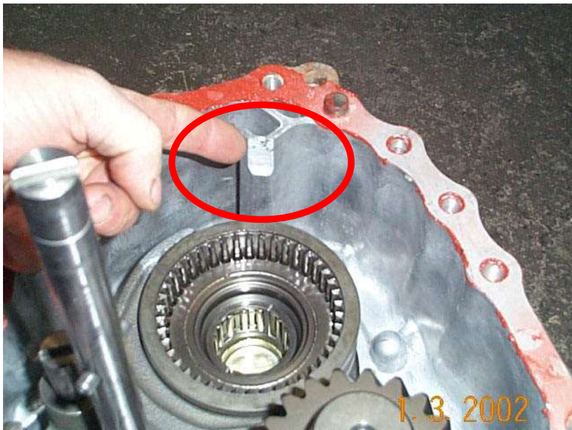
7a. Remove the front and rear bearings from the old lay shaft.
