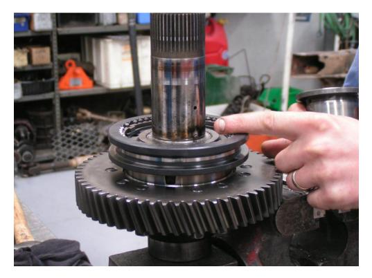
28. Re install the high range output gear, bearings and front drive gear piece. (refer page TF-27 & TF-28)
