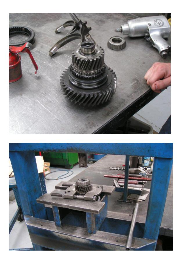
19. Remove the centre differential front drive gear piece. (refer page TF-21)
