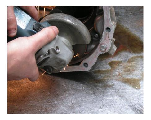
30. A small section of housing also needs to be ground away to clear the low range output gear. See the following photo.
