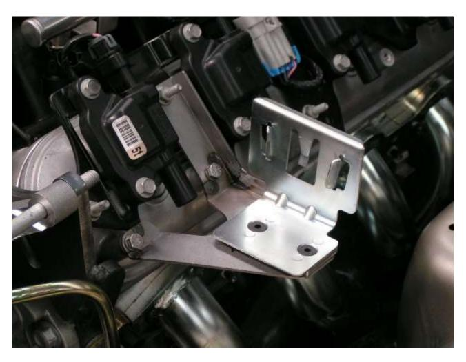
2. Fit the LS1 power steering reservoir bracket supplied in the kit. Secure it using the original coil pack bolts. See photo below:
