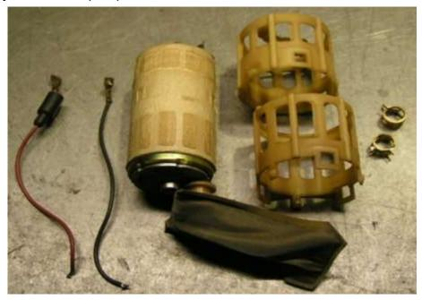
Fit the new high pressure fuel pump (GSS341).
