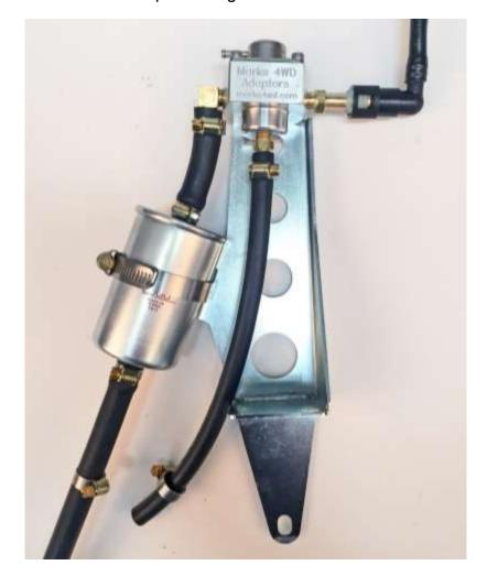
Secure the regulator with the supplied socket headed cap screws
