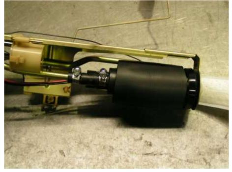
On the TB models you can blow compressed air up the fuel lines to check you have them connected correctly. Make sure you use EFI hose clamps.
