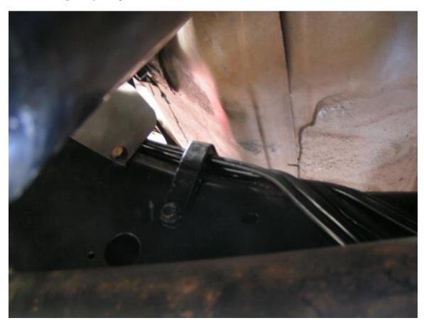
2. Secure the pipes using the original clamps. <u>Note:</u> shape of the clamps will need to be altered to secure the pipes on top of the chassis.
