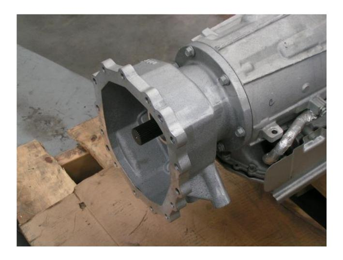
10. Fit the transfer case to the adaptor and secure it using the original bolts. *Note:* Use Threebond silicon on the mating surfaces.
