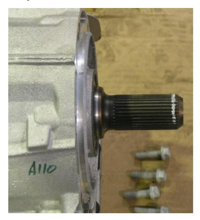
3. Cut and chamfer the output shaft at this distance.
