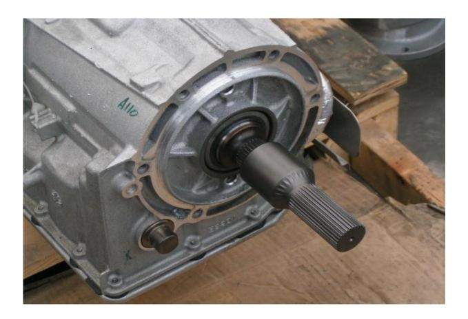
8. Fit the seal in the transfer case side of the adaptor with the spring side facing the transmission. *Note:* Use a hammer and a suitable drift.
