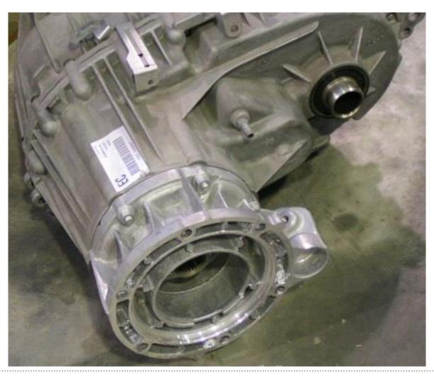
2. Measure 85mm from the rear face of the transmission and mark the output shaft. See the photo and diagram below.
