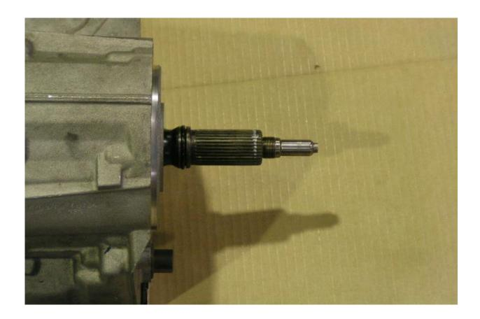
7. Check to make sure the coupler shaft fits over the previously cut and chamfered output shaft.
