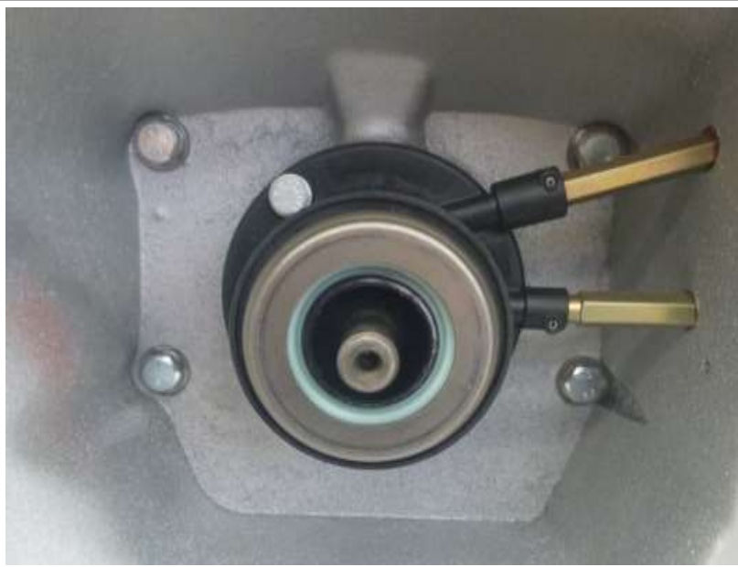
Image 3.5 Fit bell housing bolts
