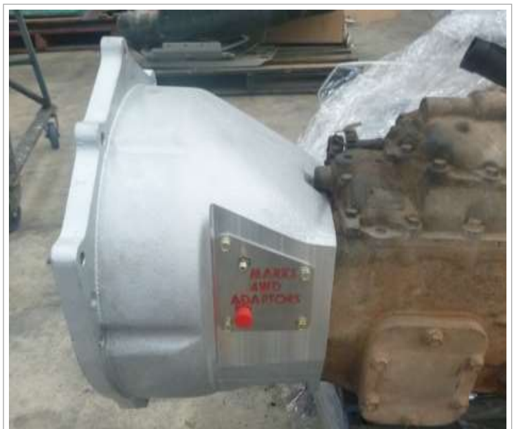
Image 3.4 Fit the new bell housing
