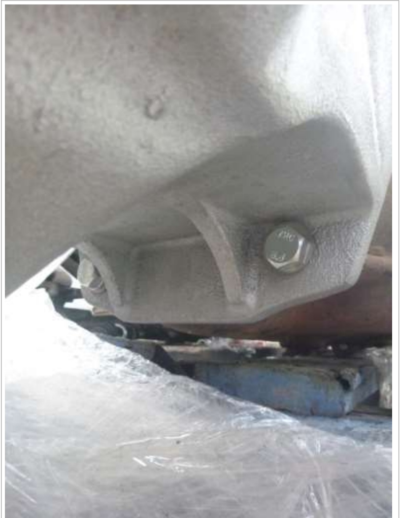
Image 3.6 Fit bell housing bolts
