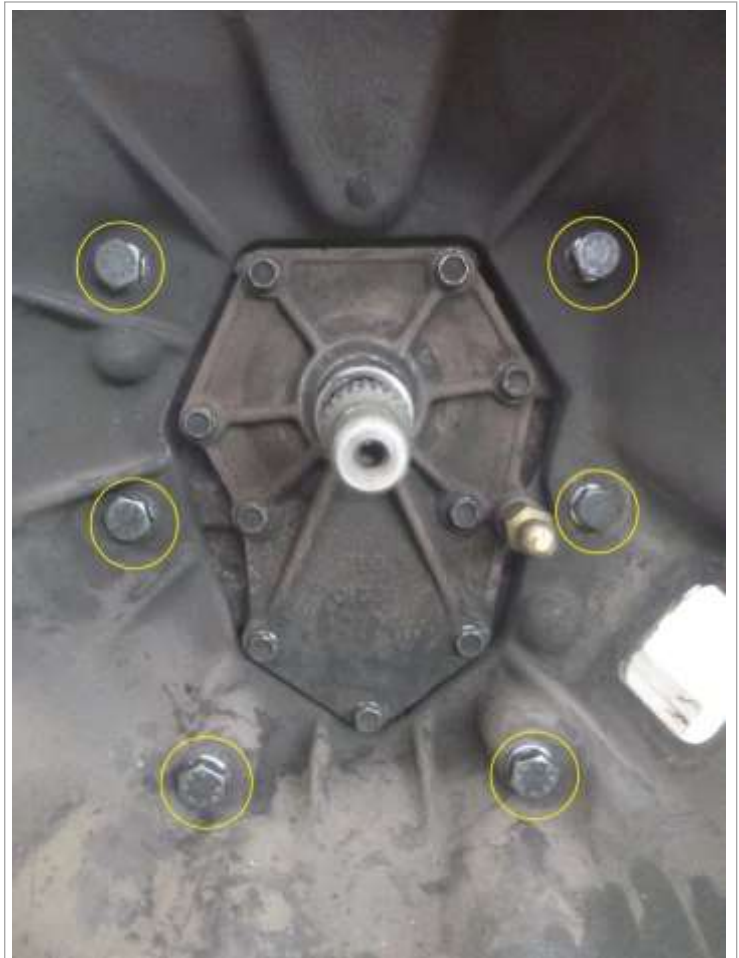
Image 1.1 Remove factory Nissan Bell Housing
