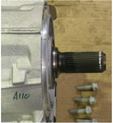
3. Cut and chamfer the output shaft as per the following diagram & photo.
