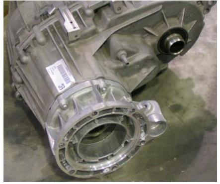
2. Measure 95mm to 97mm from the rear face of the transmission and mark the output shaft. **Note:** The 4wd transmission output shaft may not need to be cut down. See photo and diagram below.
