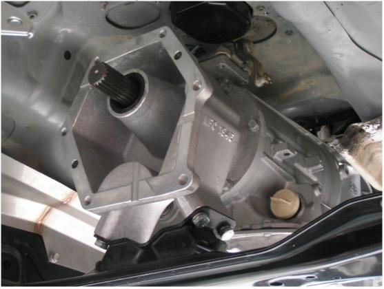
9. Fit the transfer case to the adaptor and secure it using the original bolts. **Note:** The bolt used in the centre hole on the drivers side will need to be replaced with the supplied socket head cap screw.
