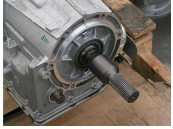
5. Fit the seal in the transfer case side of the adaptor with the spring side facing the transmission. **Note:** Use a hammer and a suitable drift.
