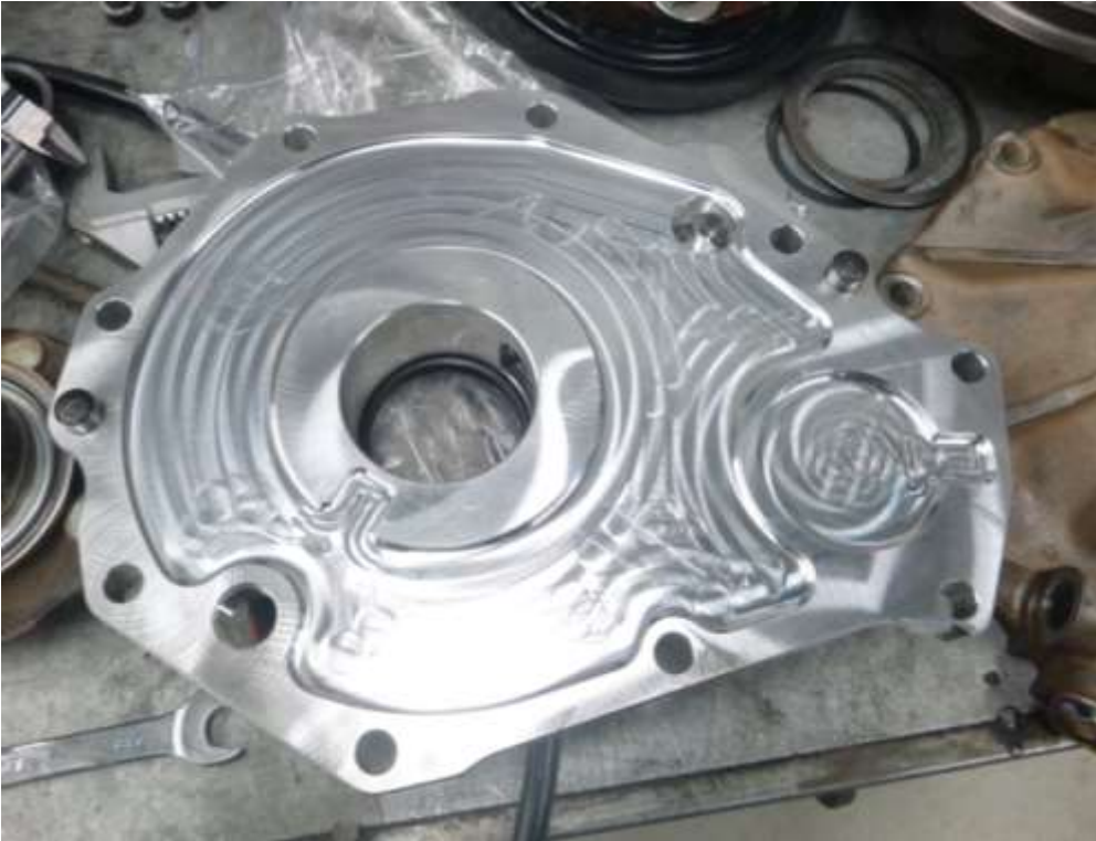
Image 2.4 Apply three bond to adaptor plate move speedo sensor
