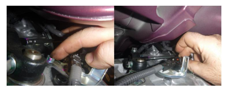
Loosen high/low switch with a 27mm spanner and carefully remove switch without damaging wiring
