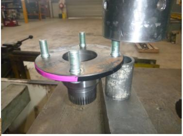
Apply Loctite 680 retaining compound to knurled area on new studs.
