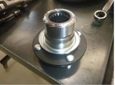
Make sure factory O-ring is positioned correctly and torque nut to 127Nm
