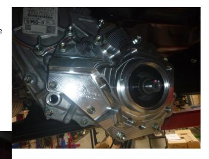
Reinstall cover bolts in their correct holes, use Loctite 263 thread locker and torque to 37Nm evenly
