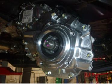
Carefully remove seal flange from output flange with a suitable prybar, work slowly around the edge as this will be reused.
