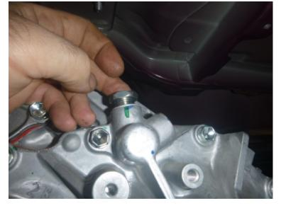
Remove top blank plug (24mm socket)
