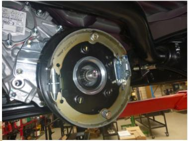
Place a small amount of oil onto rear output seal and flange area to prevent dry startup damage.
