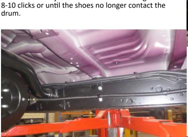
Place protective conduit on the handbrake cable and 'P' clip to chassis rail
