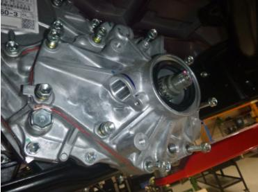
Remove 9 x M10 bolt which secure the transfer case rear cover.
