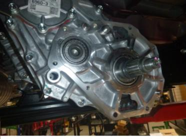
Clean the new Marks 4wd MFC20082 rear cover and carefully install the new output seal supplied into the housing with a press or similar
