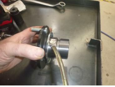
Place speedo drive gear onto output flange and reinstall onto output shaft
