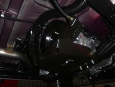
Adjust outer cable on right hand side of drum. Free play in cable to be maintained and drum should spin freely.
