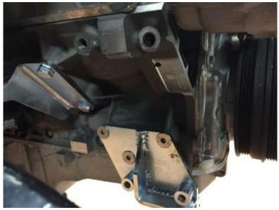
Install the top A/C bracket to the block using the x2 M10 x 1.5 x 30mm bolts and x2 M10 Spring Washers
