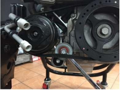
Place a 15mm ring spanner between the pulley and belt. Rotate the tensioner till it bottoms out. While holding the tensioner on its bottomed out position, slide the belt over the pulley. Release spanner off tensioner.
