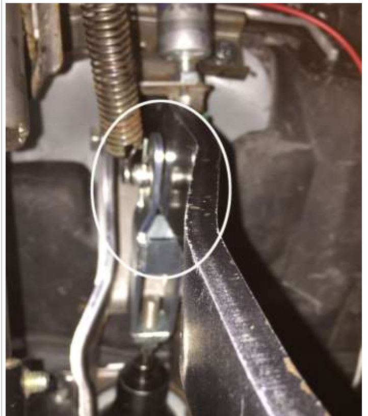
Image 3.2 Cotter pin install
