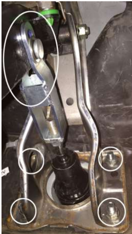
Image 3.1 Alignment of booster.
