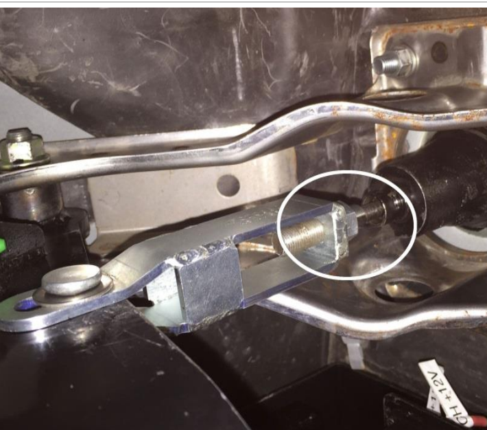
Image 3.3 Adjust the pedal saddle
