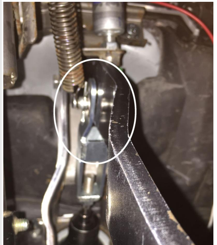
Image 3.2 Cotter pin install
