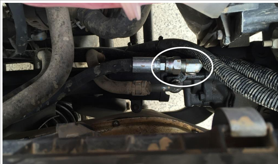
Image 4.2 Hydro boost to steering box line
