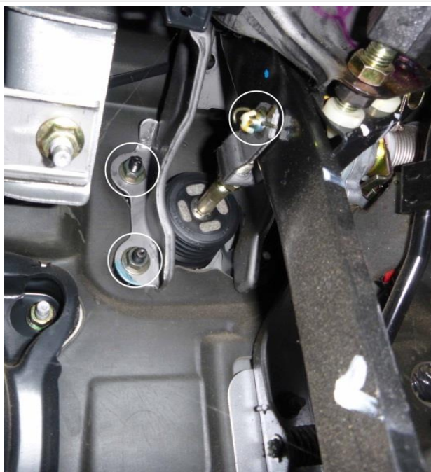
Image 1.4 Removal of the cotter pin and nuts.
