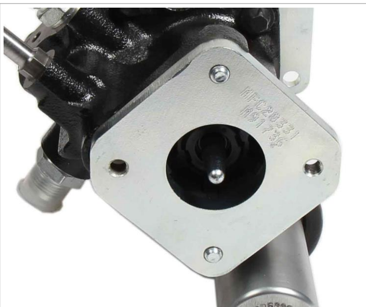
Image 2.1 Make sure the push rod is fitted in the hydro booster.
