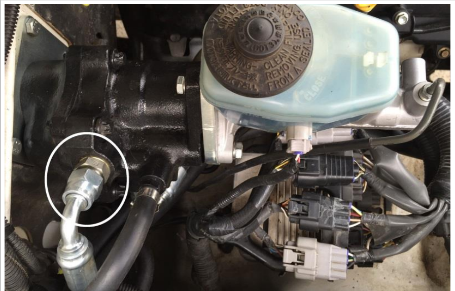
Image 4.1 Fit the master cylinder to the hydro booster
