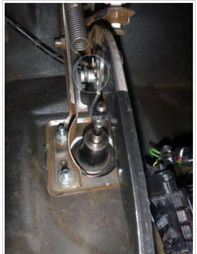
Image 3.2 Cotter pin install
