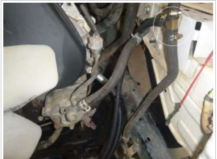
Image 4.6 Fitment to power steering resivior bottle
