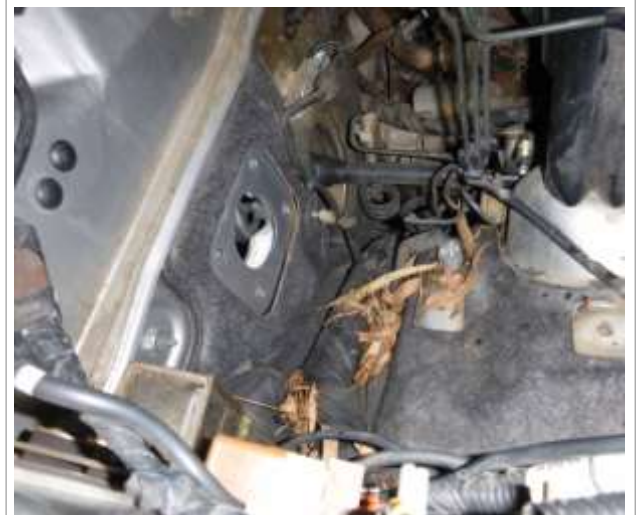
Image 1.5 Booster removed – good time to remove debris!
