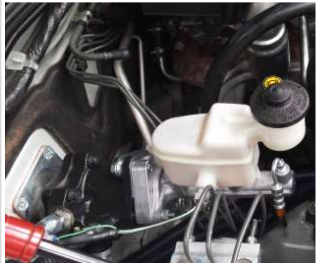
Image 1.1 Hydraulic booster setup with new master fitted
