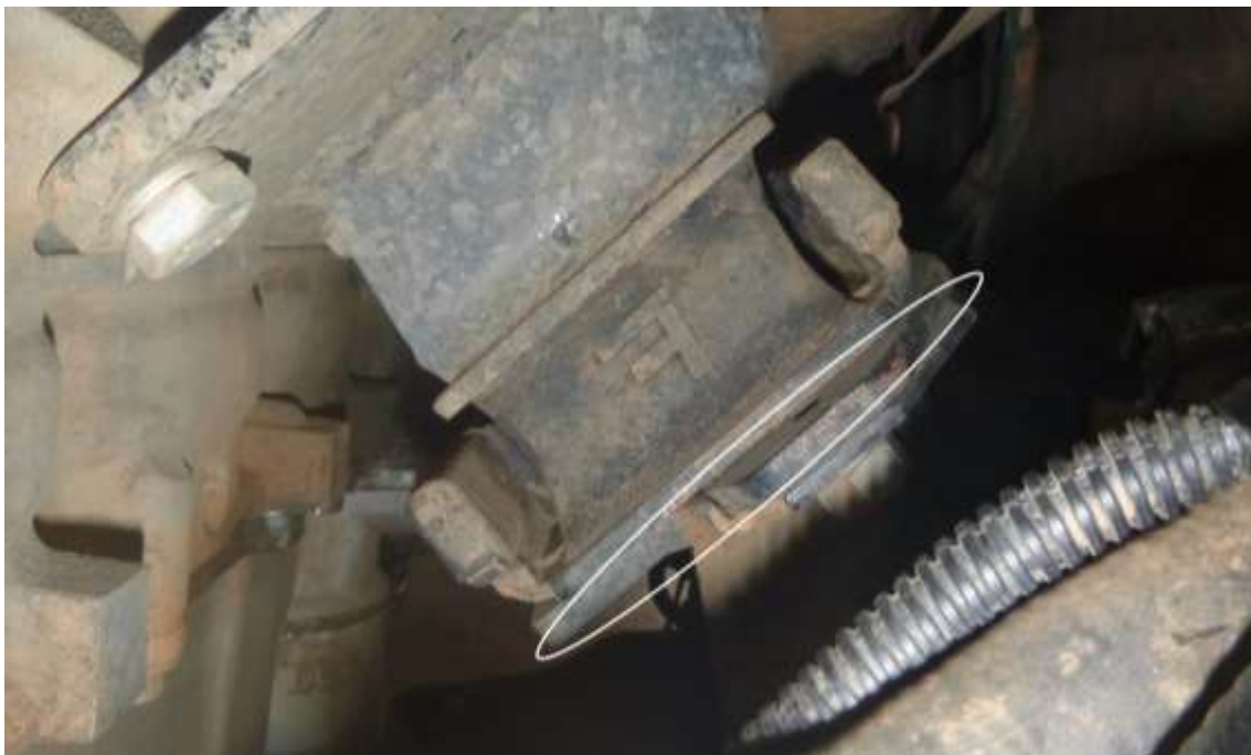
Image 1.1 Fit chassis post adaptor
