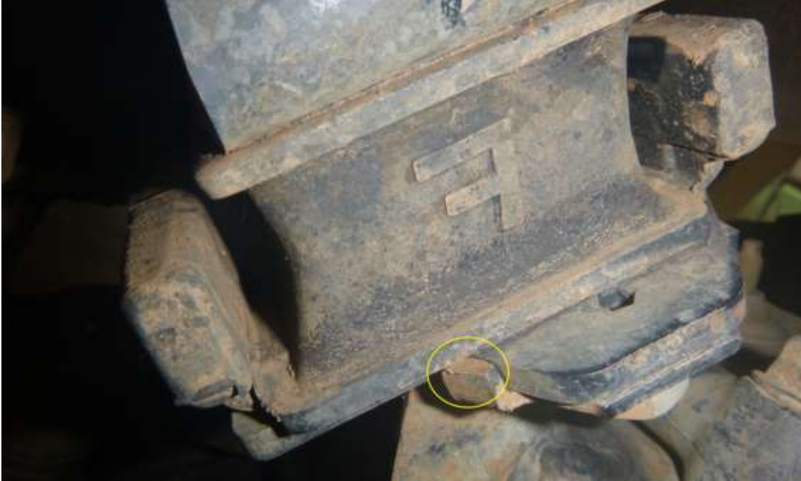
Image 1.1 Grind tabs down
