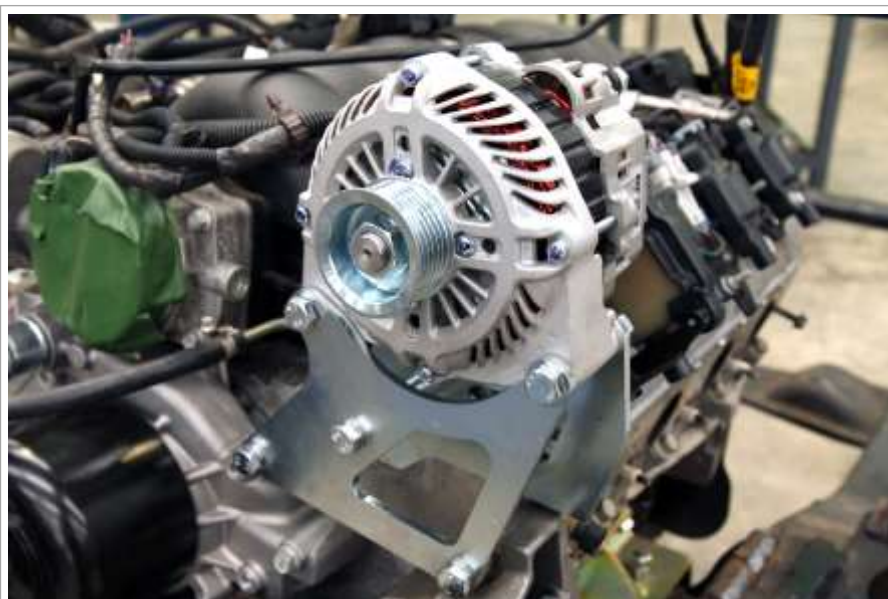
Image 4.5 Alternator mounted in the new position.
