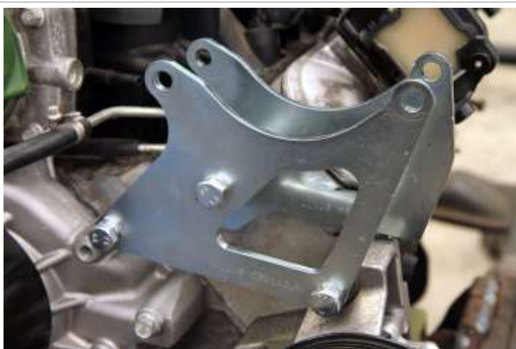
Image 4.3 Final mounting of the alternator relocation bracket
