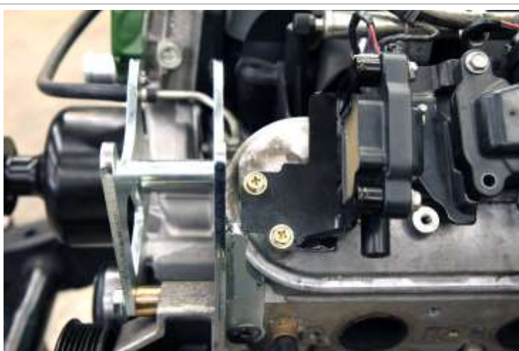
Image 4.4 Final mounting of the alternator relocation bracket
