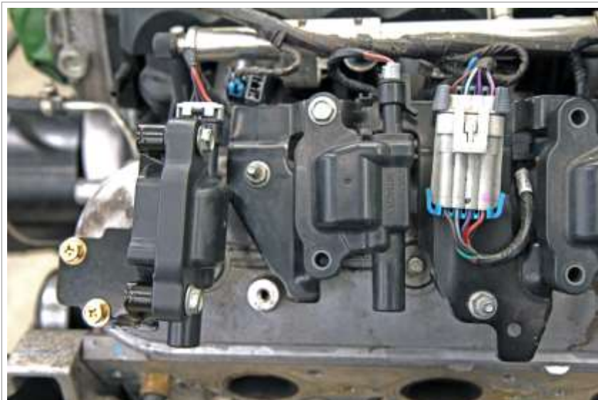
Image 2.2 Relocatoin of the 1 st ignition coil.
