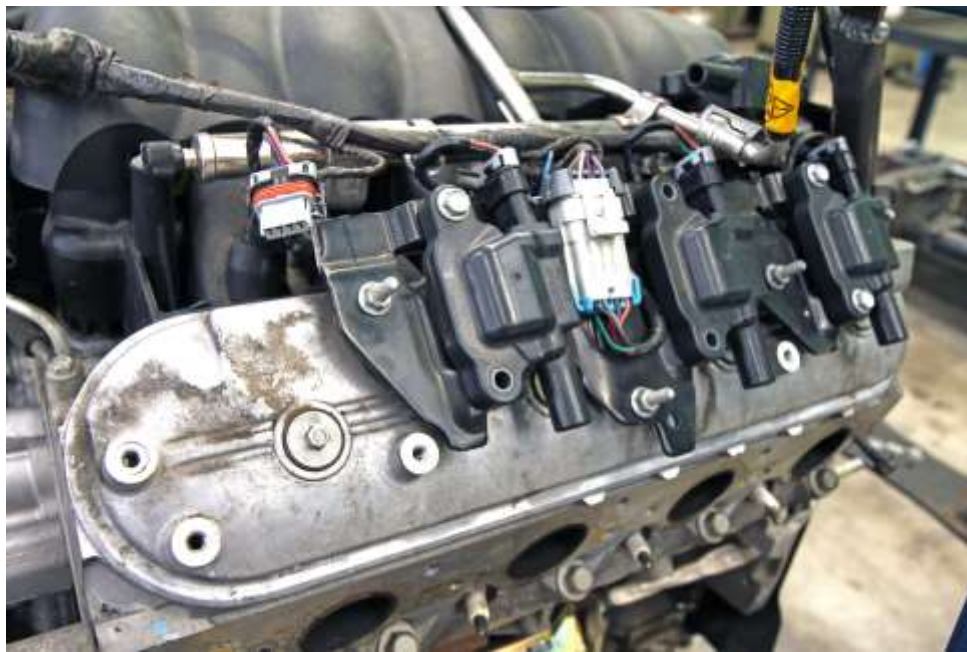
Image 1.1 Modified coil pack mount with ignition coils reattached. Note the holes where captured bolts have been left off for now.
