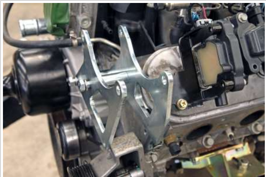
Image 4.2 The two alternator mount brackets bolted to the engine block with spacers installed.
