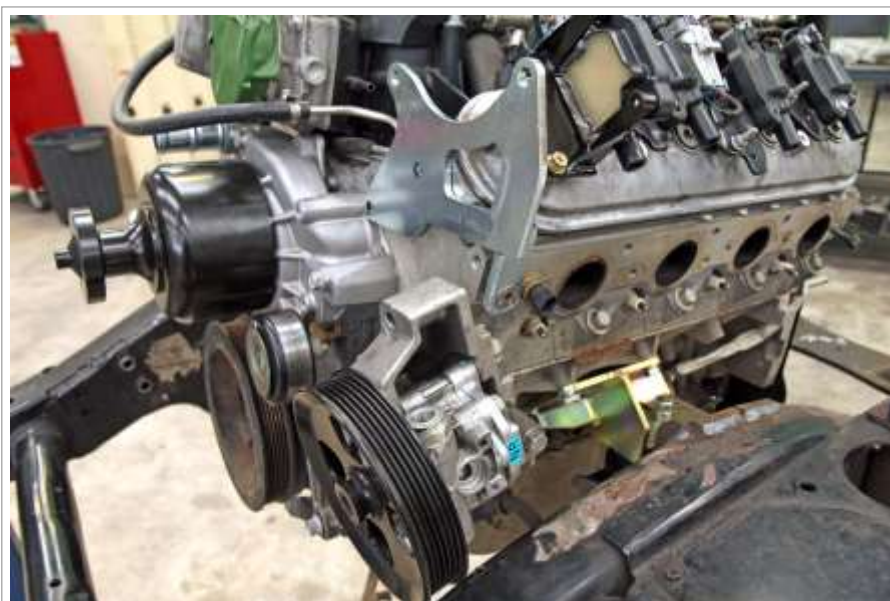
Image 4.1 Alternator relocation bracket (MFC1769) loosely bolted up.
