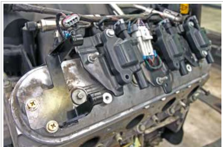
Image 2.1 Coil relocation bracket bolted to the rocker cover.
