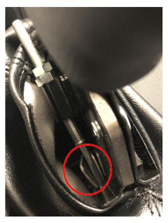
Depending on vehicle you may need to open up the handbrake guide as circled above
