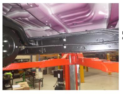
Place protective conduit on the handbrake cable and 'P' clip to chassis rail
