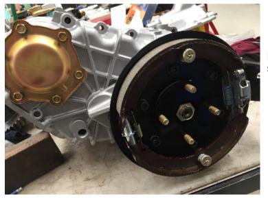
Fit the output flange with oring, fit and torque output shaft nut to 127 NM
