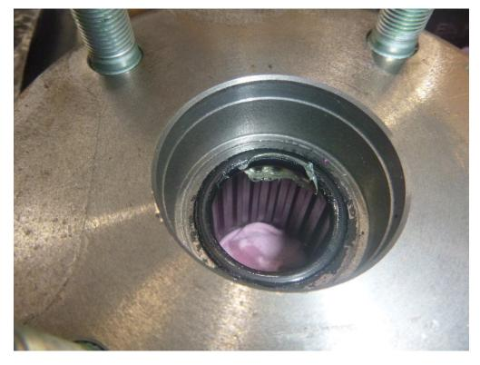
Remove the bolt, oil slinger and bearing outer cone from the bearing retainer (circled) and refit to the new bearing retainer supplied.
