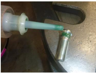
Apply Loctite 680 retaining compound to knurled area on new studs.
