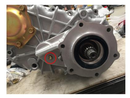
Using the supplied gasket and bolt (circled) attach new bearing housing to transfer case
