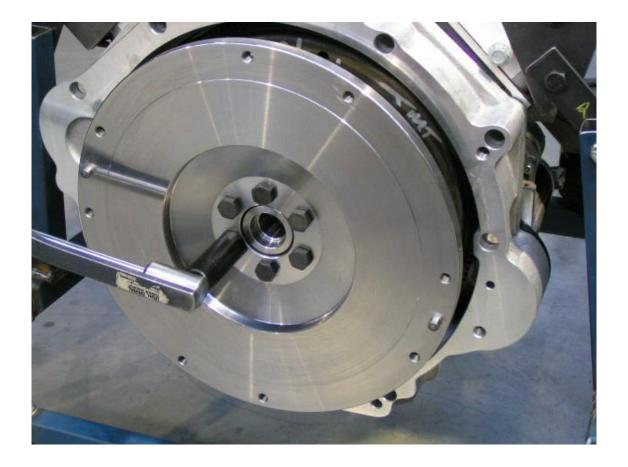
43. Fit the clutch assembly to the flywheel and secure it using the original 2F, or 3F bolts. Align the clutch plate using a suitable clutch aligning tool. NOTE: The original bolts should fit without modification but it is a good idea to double check them in the new flywheel prior to fitting the clutch.
