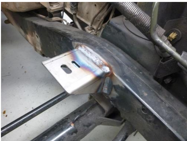
Image 1.3 Fully weld new chassis post reinforcing brackets
