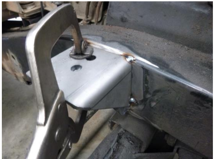
Image 1.2 Clamp the new chassis post plates in place.
