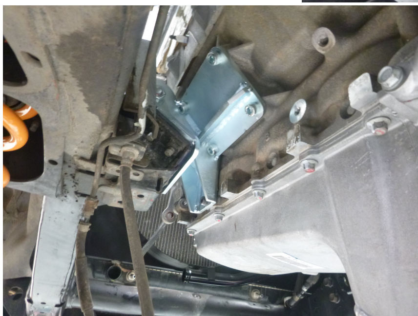
Image 1.2 M10 SHCS fitted to bracket/block
