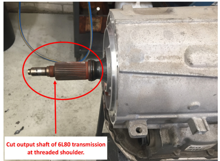
Image 2.2 Location to Cut Output Shaft 2
