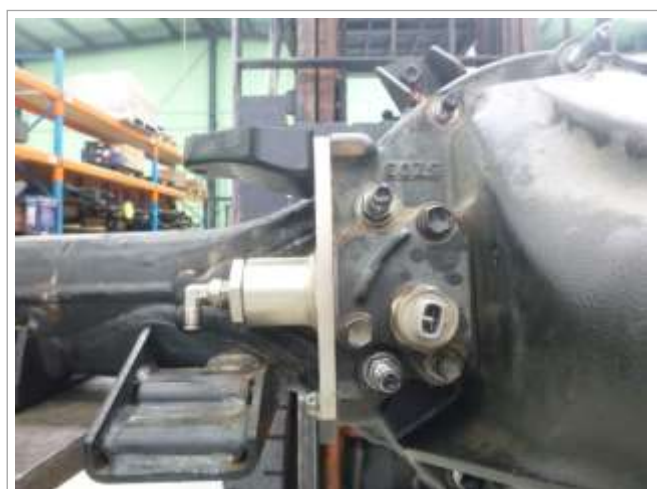
Image 5 Refit Inspection/Sensor Plate
