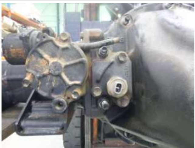
Image 2a Actuator Inspection/Sensor Plate
