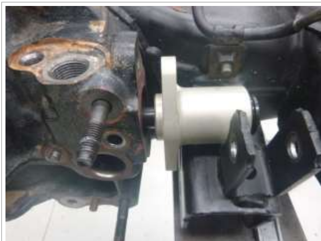
Image 10 Installing Diff Actuator
