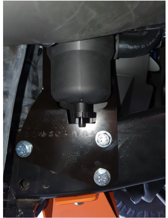
Image 6.2 Catch Can Installed
