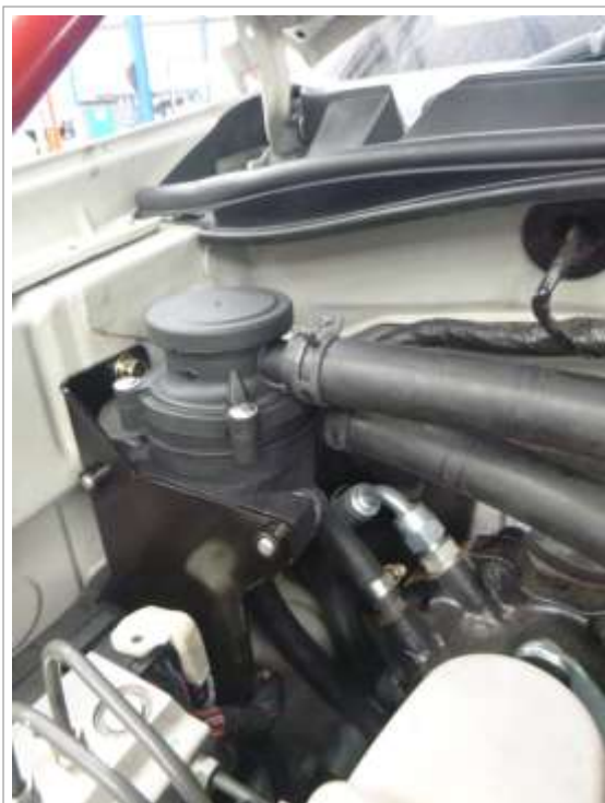
Image 3.9 Connect crank case to catch can hose
