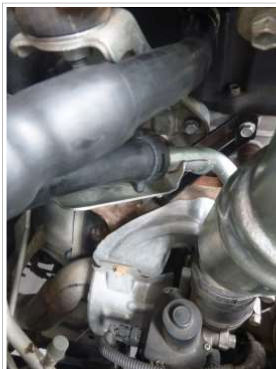
Image 3.10 Connect crank case to catch can hose
