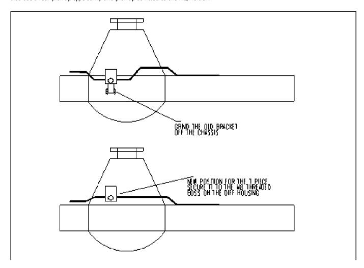
1. Remove the brake block bracket with a small grinder.
