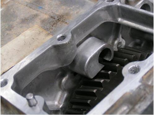
10. Remove the bearings from the old idler gear and fit them to the new one. **NOTE:** Replace the bearings if required. See following photos.
