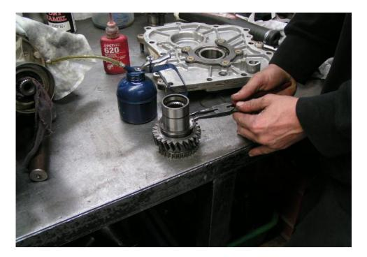
20. Re install the circlip in front of the bearing.
