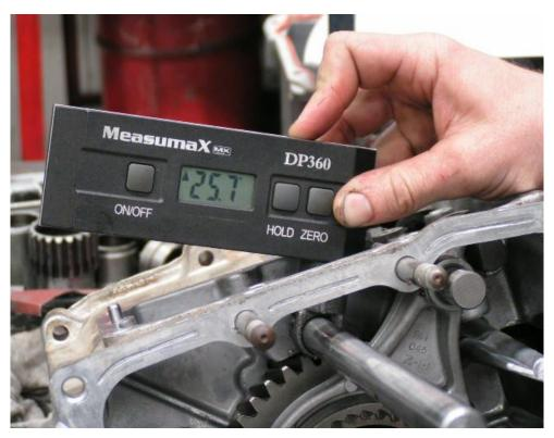
12. The gear selector can move up to 20 degrees from side to side. It's a good idea to allow a little extra clearance. See photos.
