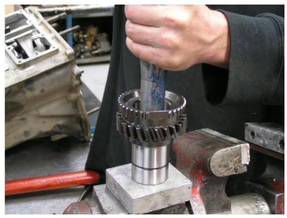
19. Slide the backlash eliminator over the input gear followed by the washer and the circlip. Then press it into the input bearing. **NOTE:** lubricate the gear, backlash eliminator and the bearing bore before fitting.
