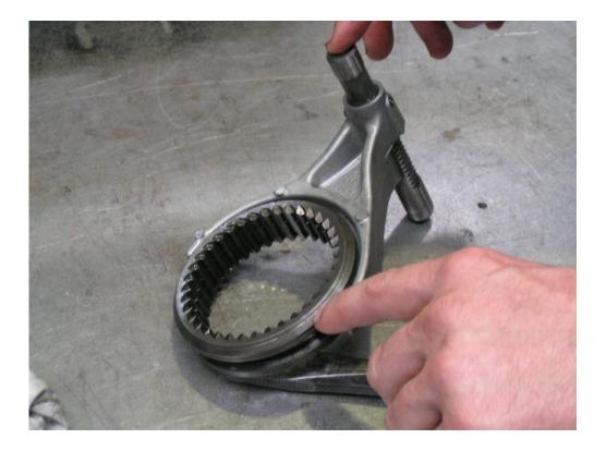
7. Remove the circlip holding the selector hub to the main output shaft. See the following photo.
