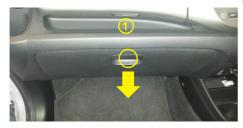
The cabin filter is located right behind the glove box. To get access to the filter it has to be removed. Follow the instructions as follows
