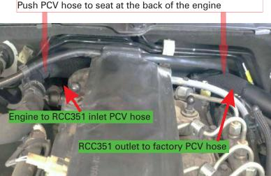
Fig 8. CATCHCAN INSTALLATION PCV HOSES LOCATIONS
