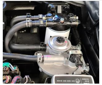
FIG. 7 FUEL WATER SEPARATOR INSTALLATION
