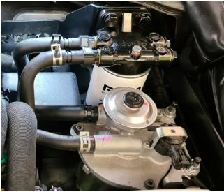
10. Start the engine and check the Z980SK16 fuel filter, fittings and hoses for any leaks.
