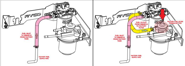
FIG. 6 FUEL INLET HOSE ROUTING
