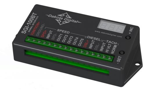
Setup menu overview \*To simplify the setup procedure, please download out IOS or Android app 'Dakota Digital Accessory'\* Setup is entered by holding the SET switch while turning the key on. The INC switch is used to change selections and the SET switch is used to save or select.
