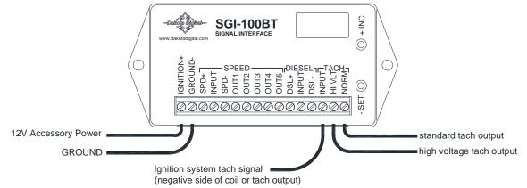
Note: If the TACH NORM output does not drive your tachometer, use TACH HI VLT.
