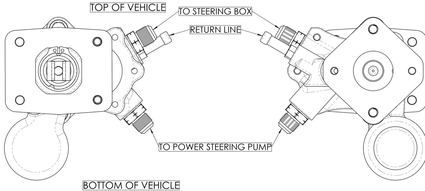
NOTE: RETURN LINE SHOULD BE "T" IN AS CLOSE TO POWER STEERING RESERVOIR AS POSSIBLE
