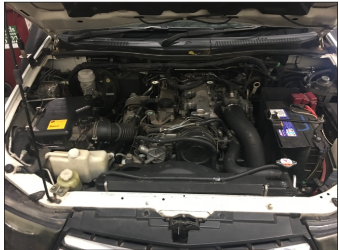
FIG.11 ENGINE COVER REMOVED
