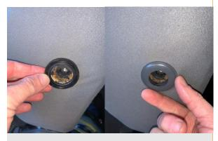
**4.** Insert inner cloth clip behind seat fabric, then place outer cloth clip (colour matched to arm rest) over the top and clip the two parts together.
