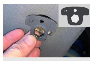
**3.** Insert plate marked "LF" through the hole, the overhanging shoulders will rest atop the upright bracket. The nut on the seat should be evident through the hexagon slot on the plate.
