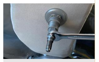
**6.** The inner stud can then be fitted and secured to the captive nut in the seat bracket. Tighten firmly into position using **10mm Open Ended Spanner**.
