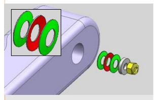
**9.** The arm rest can now be bolted up, please note the orientation of the spring washers as shown, followed by the supplied flat washer and nut.
