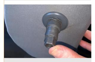
**5.** Insert the outer shaft into the plate, it is essential that the hexagonal end of the shaft slots into the hexagonal slot in the plate.
