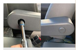
**10.** Use a **13mm Socket** to tighten the nut firmly into position. Once the arm rest is bolted In, the end cap can be installed to complete the installation.
