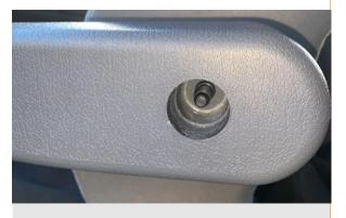
**8.** The arm rest can then be installed (the orientation of the armrest on the shaft will set the lowest tilt adjustment point of the armrest).
