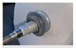
**7.** The inner arm rest cap can be placed on the shaft as shown.
