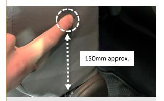
**1.** Feel the side of the seat for a bolt head (in the vicinity of 150mm from the plastic trim on the side of the seat as shown).
