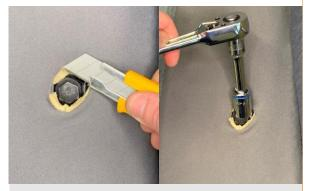
**2.** Using a sharp utility knife or similar, make a hole around the bolt head big enough for the supplied mounting plate to pass through. Use a **14mm Socket** to remove the existing bolt from seat frame.
