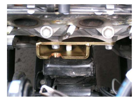
Tighten all of the engine mounting nuts and bolts.
