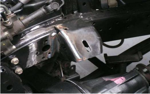
Complete the welding of the bracket and grind of any access weld. Re-paint the chassis rail and mounting. Re-install the steering box mounting bolts.
