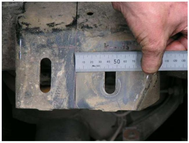
As shown in the photo above, mark a line on the bracket 35mm from the front edge of the rear slot. This line should go all the way back to the weld on the top of the chassis. The white line on the left of the photo should also be marked back to the chassis. The section you remove should be 65mm wide.
