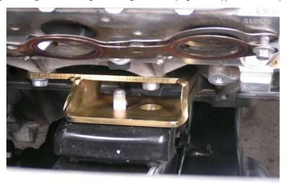
Install the Toyota engine mounting rubber. **NOTE:** The top stud on the passenger side mount will need to be cut down by approximately 10mm. See photo below.
