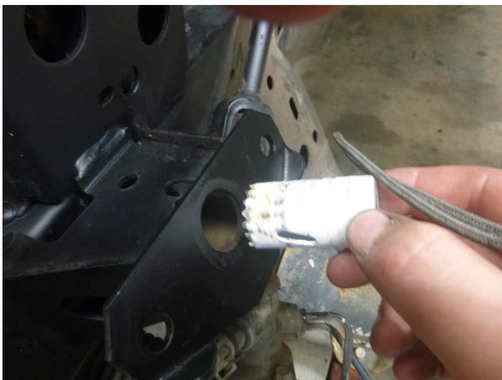
Image 4.1 Drill Toyota Chassis Post
