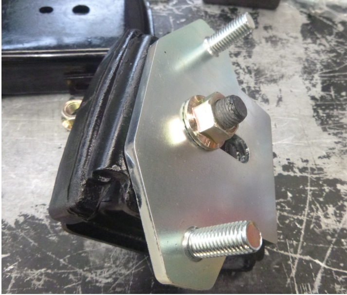
Image 5.1 Rubber mounts to chassis post bracket
