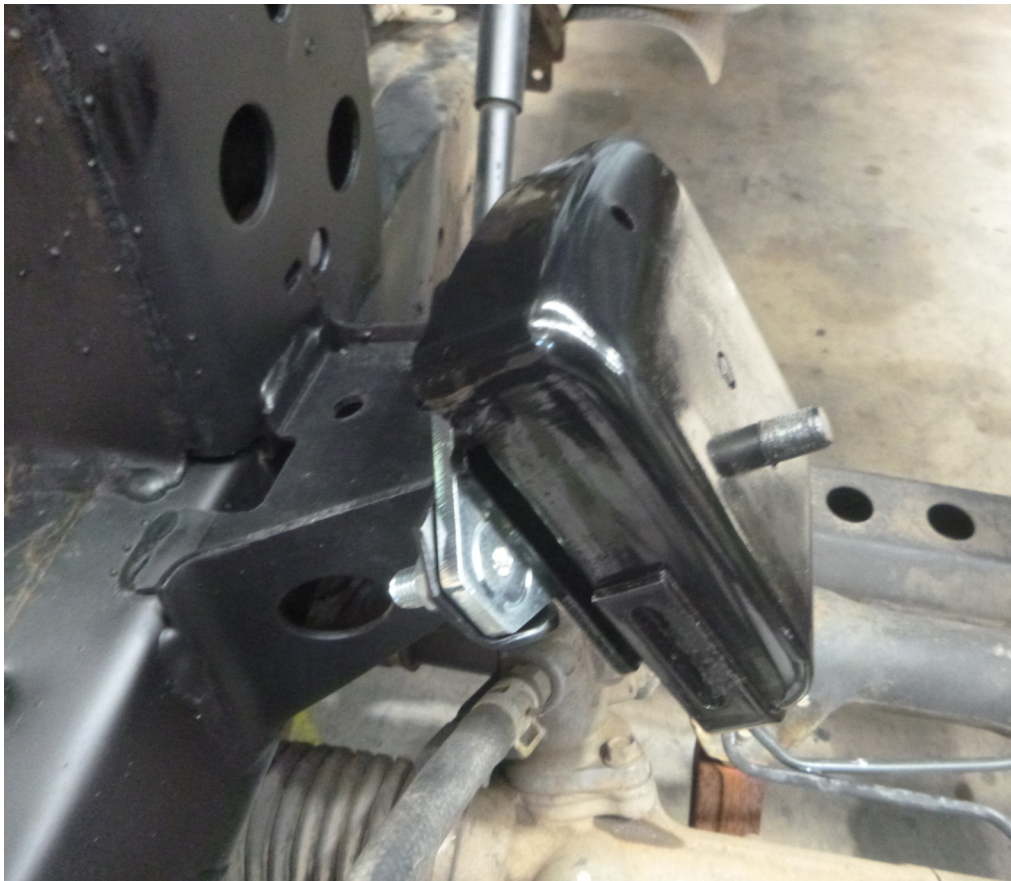
Image 5.3 Assembled to RHS chassis post
