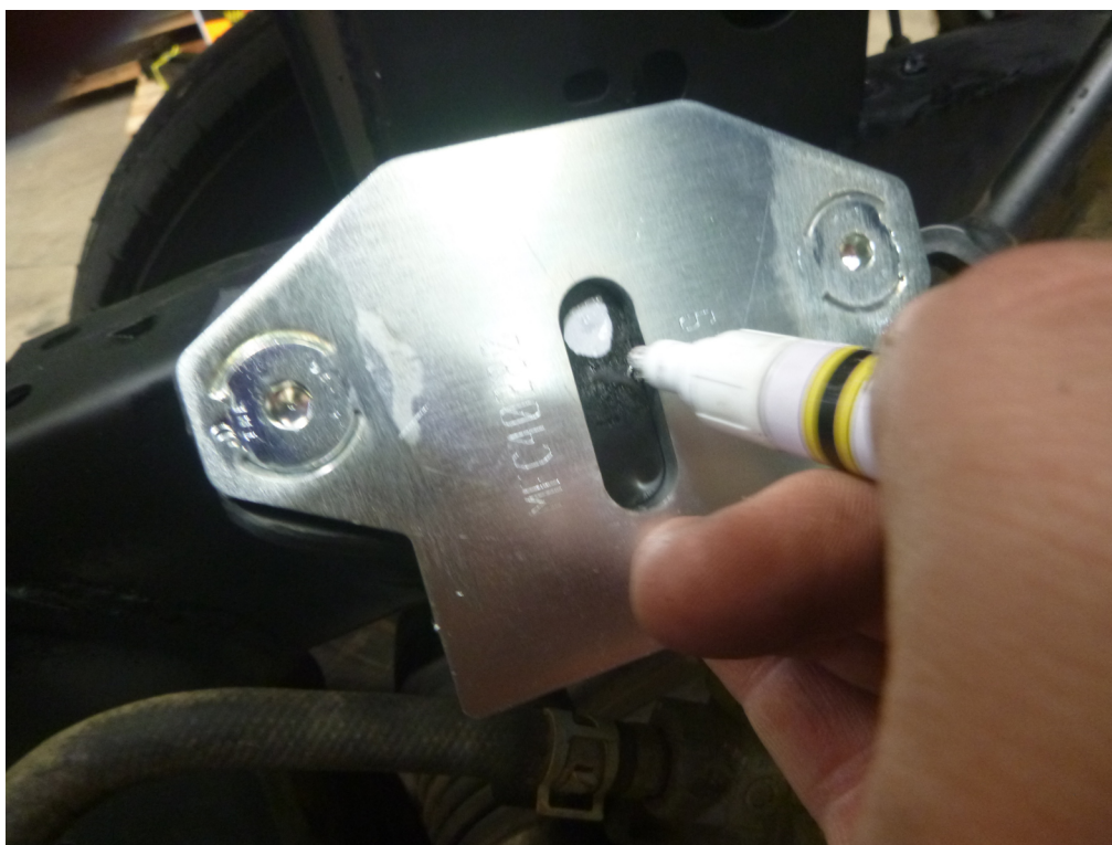
Image 3.1 Marking Chassis Post
