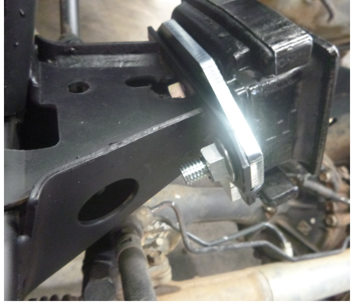
Image 5.2 Bolted to chassis post
