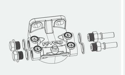
**FIGURE 3** FUEL WATER SEPARATOR HEAD PREPARATION
