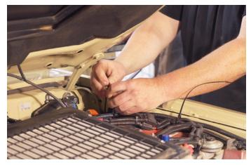
4 Then, run the positive and negative wires to the battery.
