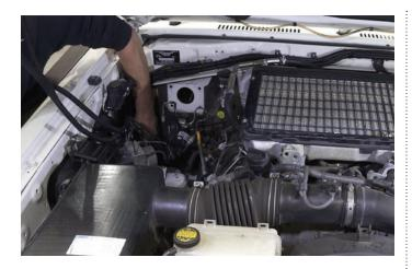
3 You will then be able to run the wiring harness through the engine bay using cable ties where possible to ensure that they are secured away from any moving parts or heat sources.
