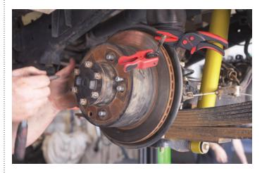
Once the rear rotors have been machined or replaced, fit the new Bendix Ultimate 4WD Brake Pads (DB1200) and brake pad mounting hardware over to the new Bendix caliper, making sure to use Bendix Ceramasil Brake Parts Lubricant where needed, and fit the caliper to the vehicle.
