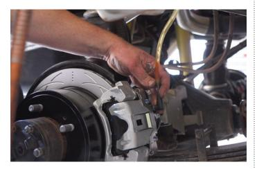
Be sure to secure the caliper wiring up and away from any moving parts using cable ties.
