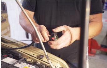
Then, connect the Red AC Wire with green trace on the wiring plug to the ignition switch.
