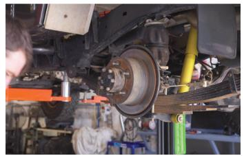
Begin by running the Electric Park Brake caliper wires along the chassis rail down to the differential and out to each caliper. Be sure to secure the harness to the chassis rail using cable ties at various points.
