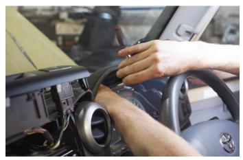
Cocate the same colour wire and confirm using a multimeter. Once confirmed, connect the LED Vehicle Park Brake Dash Light Wire to the identified wire.
