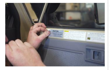
The Ultimate 4WD EPB also has a 'service mode' to wind back the EPB to allow for brake pad change. There is a card detailing this process provided within the kit. Be sure to add this to the vehicle service book so future service technicians can understand this process.
