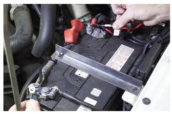
To test operation, turn the ignition off and with the OEM hand brake disengaged, check that the Electric Park Brake activates, and the Vehicle Park Brake Dash Light comes on.
