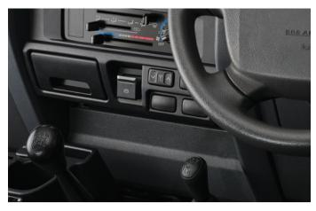
9 For the Workmate variant without electric mirrors, the switch can be fitted to a blanking plate on the dash to the right-hand-side of the steering column. Once the provided switch has been mounted in the preferred position, connect the wiring into the switch.
