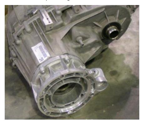
2. Measure 95mm to 97mm from the rear face of the transmission and mark the output shaft.
