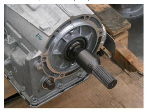
5. Install the seal in the transfer case side of the adaptor with the spring side facing the transmission. **Note:** Use a hammer and a suitable drift.
