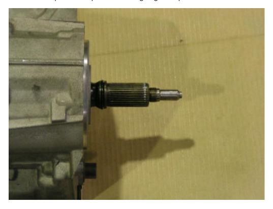
4. Check to make sure the coupler shaft fits over the previously cut and chamfered output shaft
