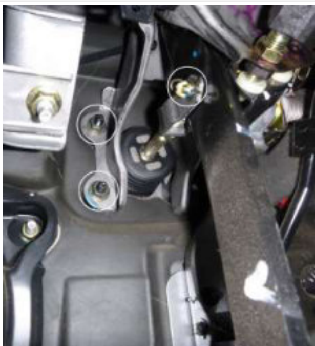
Image 1.4 Removal of the cotter pin and nuts.
