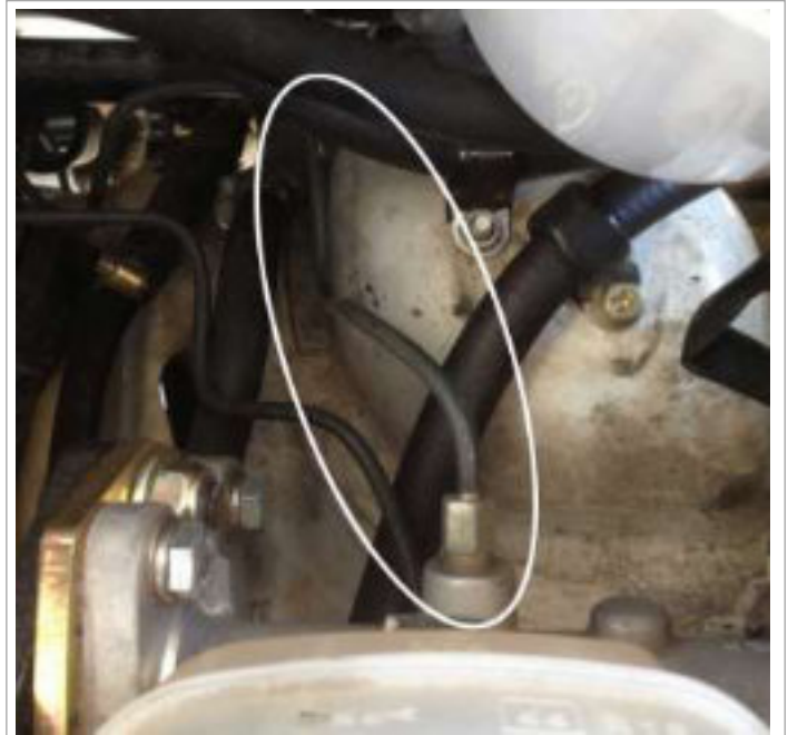
Image 5.2 Connect the factory Nissan hard line to the master
