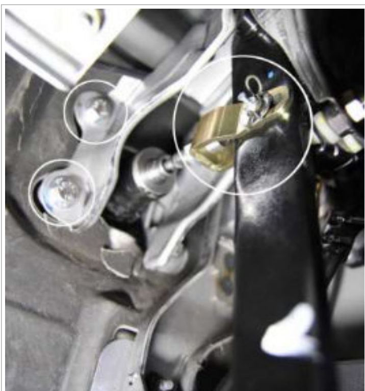
Image 3.1 Alignment of booster.
