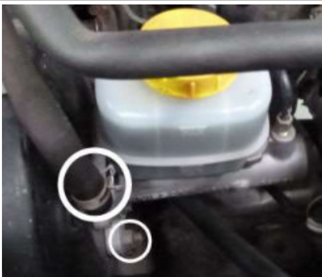
Image 1.2 Removal of 4 nuts & vacuum pipe.
