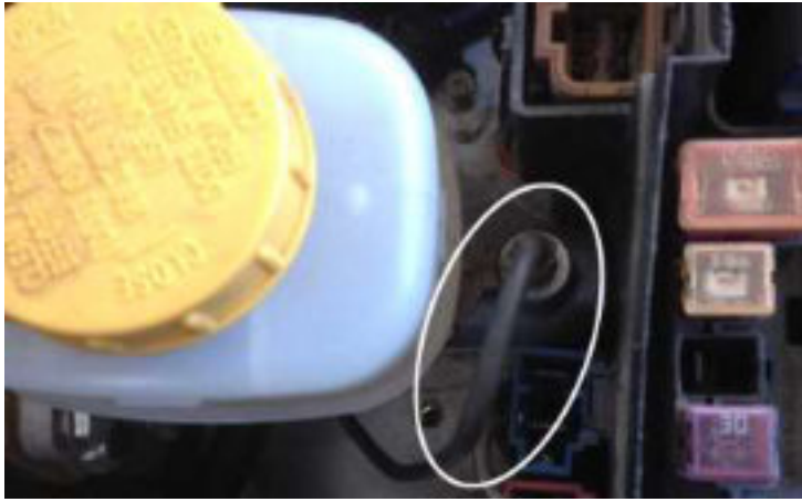
Image 5.1 Connect the factory Nissan hard line to the master
