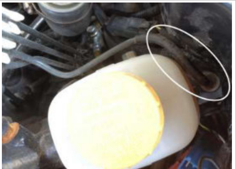
Image 5.3 Connect the factory Nissan hard line to the master
