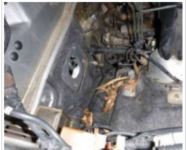
Image 1.5 Booster removed – good time to remove debris!
