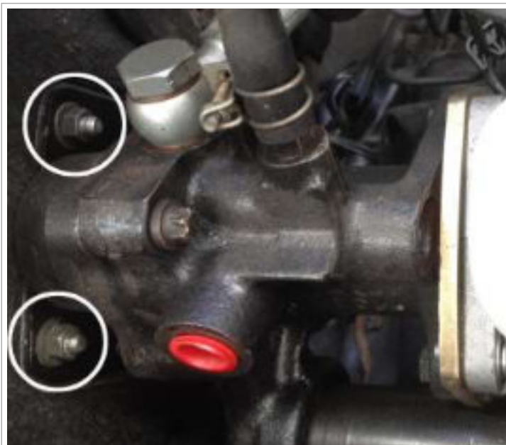
Image 3.3 Fit the factory M8 nuts to the bolts
