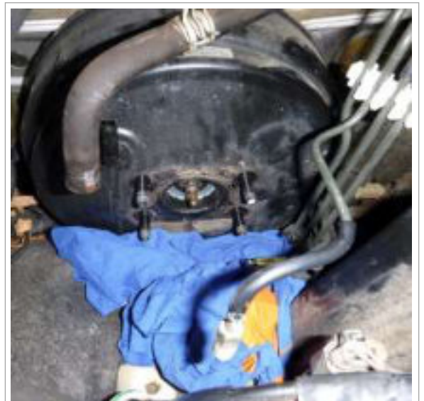
Image 1.3 Removal of 4 nuts & vacuum pipe.
