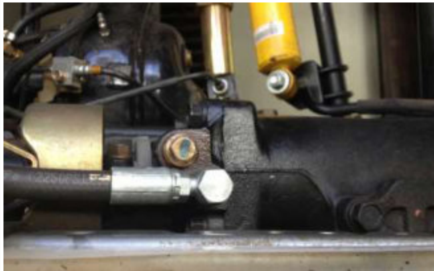
Image 4.2 Hydro boost to steering box line
