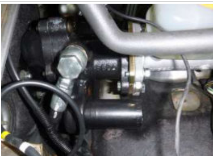
Image 4.3 Booster to power steering pump
