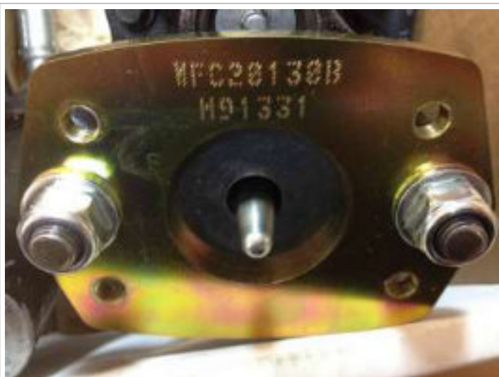
Image 2.1 Make sure the push rod is fitted in the hydro booster.
