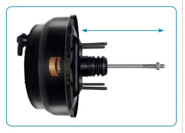
On the original booster, measure the distance from the fire wall face to the pedal mount and adjust the new booster to the same length.
