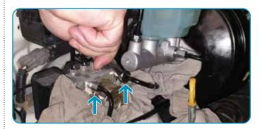
4 With **ignition off** remove any air caught in the pipes between the master cylinder and ABS pump. Using a pipe spanner, loosen the fitting on the ABS pump while another person gently applies the brake pedal. Do not let the master cylinder reservoir run out of brake fluid when bleeding. Brake fluid and any air should come out of the fitting. Tighten the fitting before brake pedal is released.
