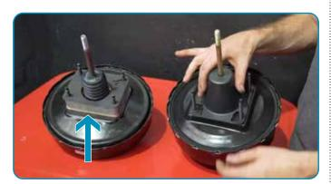
2 Install the master cylinder making sure the push rod end is mated squarely with the master cylinder. Adjust the position of the brake pipes as required then re-install brake pipes and vacuum hose.
