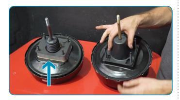
Place the supplied gasket onto the booster. Guide the pushrod through the firewall, inside the vehicle, ensure the pushrod is correctly guided onto the pedal.
